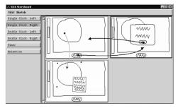
**Figure 1.** A storyboard window in SILK with more event types. The arrows pointing left and right represent left single click, and the arrow pointing down represents right single click. In the prototype, the arrows are different colors.
